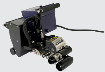
The robust and reliable Weldy hot-wedge welding machine, WGW 300, is suitable for safely welding geomembranes inmines, landfills, ponds, fish breeding basins etc.
